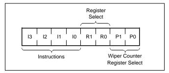
The four high order bits define the instruction. The next two bits (R1 and R0) select one of the four registers that is to be acted upon when a register oriented instruction is issued. The last bits (P1, P0) select which one of the four potentiometers is to be affected by the instruction.
