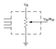
Three terminal Potentiometer; Variable voltage divider
