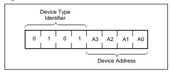
The next four bits of the slave address are the device address. The physical device address is defined by the state of the A0 - A3 inputs. The X9258 compares the serial data stream with the address input state; a successful compare of all four address bits is required for the X9258 to respond with an acknowledge. The  $A_0$  -  $A_3$  inputs can be actively driven by CMOS input signals or tied to  $V_{CC}$  or  $V_{SS}$ .
