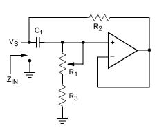
$Z_{IN} = R_2 + s R_2 (R_1 + R_3) C_1 = R_2 + s Leq (R_1 + R_3) >> R_2$
