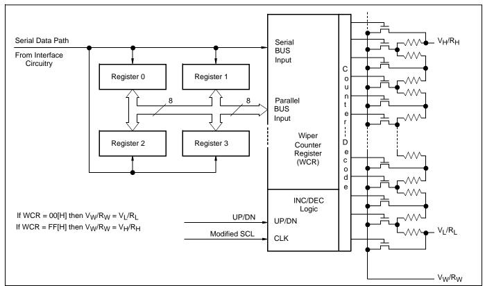
All DCP potentiometers share the serial interface and share a common architecture. Each potentiometer has a Wiper Counter Register and four Data Registers. A detailed discussion of the register organization and array operation follows.
