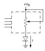
Two terminal Variable Resistor; Variable current
