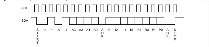
The Increment/Decrement command is different from the other commands. Once the command is issued and the X9258 has responded with an acknowledge, the master can clock the selected wiper up and/or down in one segment steps; thereby, providing a fine tuning capability to the host. For each SCL clock pulse ( $t_{\mbox{HIGH}}$ ) while SDA is HIGH, the selected wiper will move one resistor segment towards the  $V_{\mbox{H}}$  terminal.
