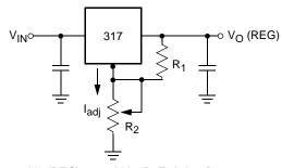
$V_{O}(REG) = 1.25V (1+R_2/R_1)+I_{adj} R_2$
