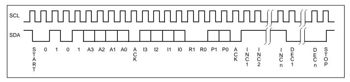
Figure 6. Increment/Decrement Timing Limits
